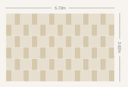
20.74m² two size mixed paving laying guide (Approx size: 5730 x 3620mm)
